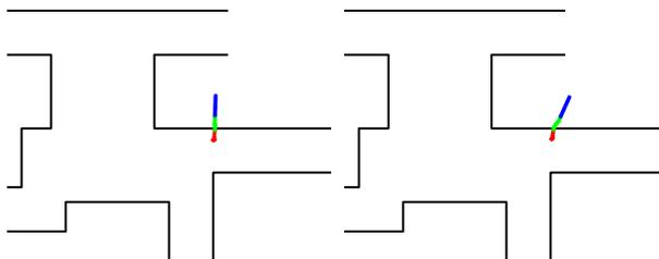
Figure 10: Some atypical gestures are actually illusions caused by sensor failures. These examples were generated by system initialization transients.
