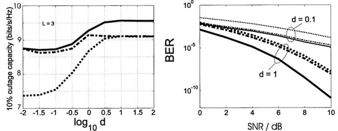
Fig. 2. Left graph: 10% outage capacity with respect to the relative antenna spacing  $d$  for  $\rho = 20$  db. Right graph: BER of BPSK as a function of SNR for  $d = 0.1$  and  $d = 1$ . Full-complexity receiver (solid curve), pure antenna selection (dotted curve) and FFT-antenna selection (dash-dotted curve) with  $t = 2$ ,  $r = 8$ ,  $\theta_r = (\pi/4)$  and  $\sigma_r = (\pi/12)$ . with same channel and system parameters.
