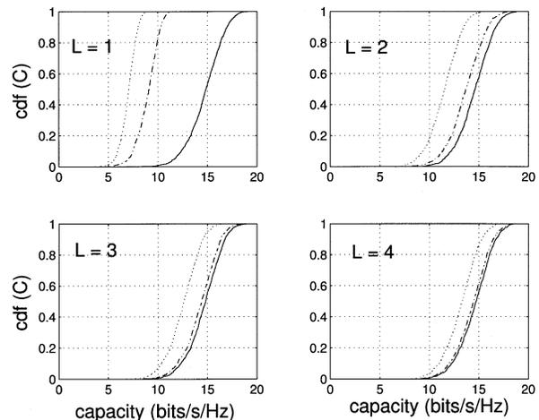
Fig. 5. Capacity cdf with spatial multiplexing: full-complexity (solid curve), antenna selection (dotted curve) and beam selection (dash-dotted curve) with  $t = 2$ ,  $r = 8$ ,  $\rho = 20$  dB,  $d = 0.5$ ,  $\theta_r = (\pi/12)$  and  $\sigma_r = (\pi/12)$ .
