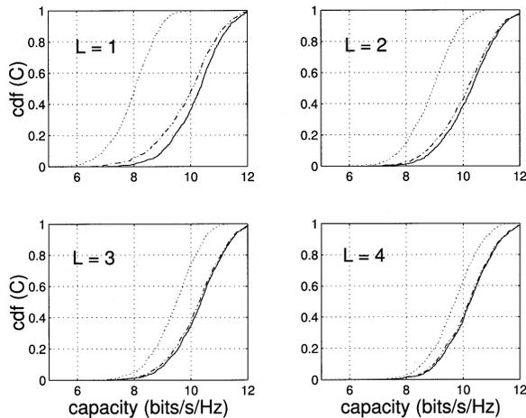
Fig. 3. Capacity cdf: full-complexity system (solid curve), pure antenna selection (dotted curve) and FFT-antenna selection (dash-dotted curve) with  $t = 2$ ,  $r = 8$ ,  $\rho = 20$  dB,  $d = 0.5$ ,  $\theta_r = (\pi/12)$  and  $\sigma_r = (\pi/12)$ .
