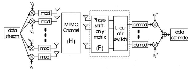
Fig. 1. MIMO channel model and system diagram.
