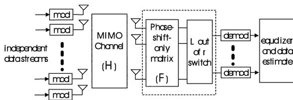
Fig. 4. System and channel model for spatial multiplexing.
