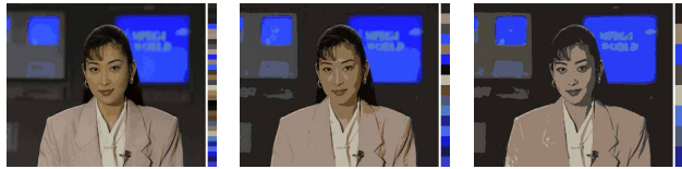
Fig. 4. Quantization by 32, 16, and 8 dominant colors, which are shown next to each image. As visible, very low quantization levels may disturb the color properties, i.e. skin colors and edges.
