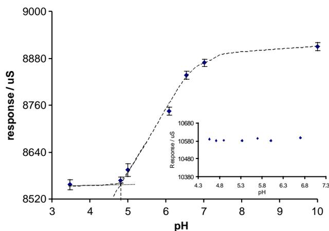
Fig. 7. Response of the fused-LEDs optical probe to a change in pH of 1.85  $\mu\text{M}$  BCP solution. Each data point represents an average of three repeats and the error bars represent the standard deviation. Inset: Response of fused-LEDs optical probe to a change in pH of water acidified with HCl to pH 3.
