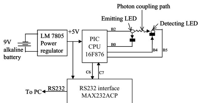
Fig. 2. Block diagram of circuitry used for the optical probe.
