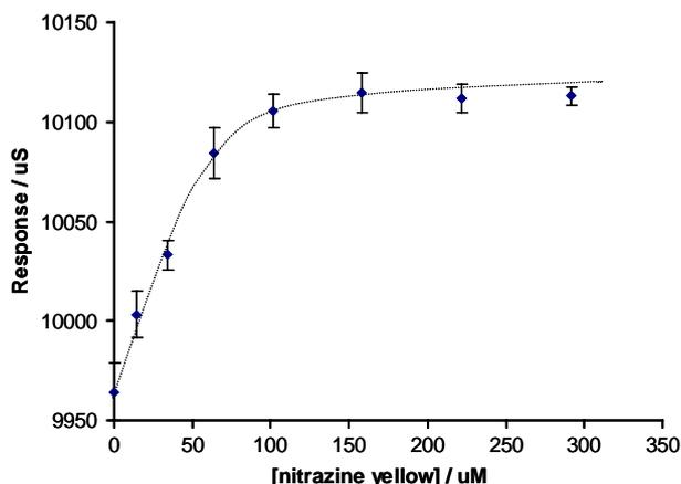
Fig. 4. Response of the fused-LEDs optical probe to a change in nitrazine yellow concentration. Each data point represents an average of three repeats and the error bars represent the standard deviation. The dotted line acts only as a visual aid.
