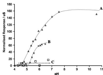
Fig. 8. Effects of ethylene glycol to pH titration of (A) BCP dye solution, (B) mixture of BCP + EG and (C) EG only.
