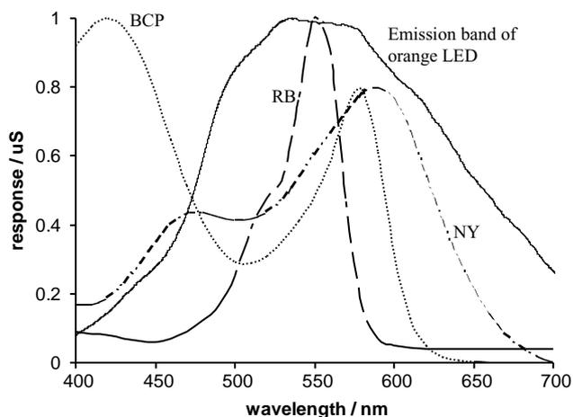
Fig. 3. Emission spectrum of LED used in optical probe and the absorption spectra of nitrazine yellow (NY), rhodamine B (RB) and bromocresol purple (BCP).
