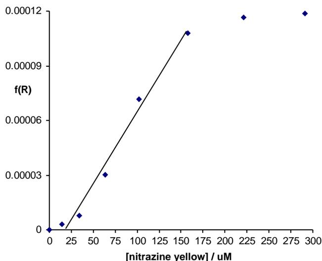
Fig. 6. The Kubelka–Munk function  $f(R)$  vs.  $C$  plot obtained with the fused-LED sensor probe and nitrazine yellow.
