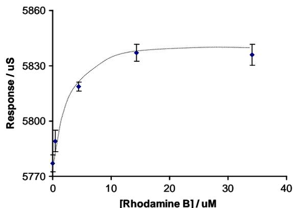
Fig. 5. Response of the fused-LEDs optical probe to a change in rhodamine B concentration. Each data point represents an average of three repeats and the error bars represent the standard deviation. The dotted line acts as a visual aid.
