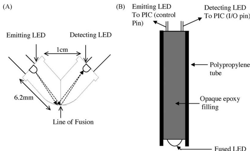
Fig. 1. Schematic of (A) a fused-LEDs and (B) cross-section of the optical probe.
