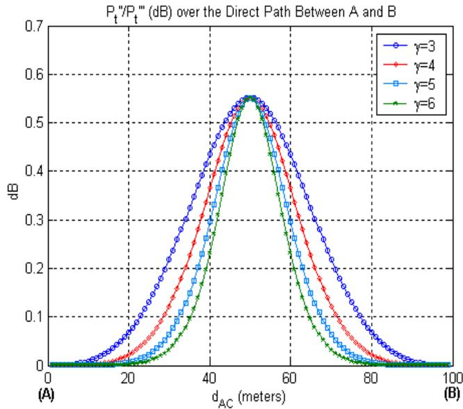
Figure 5 Power savings of regenerating with respect to simple relaying at intermediate node positions over the direct path between A and B separated with 100m.
