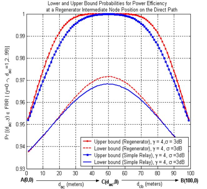
Figure 2 Illustration of the probability of an intermediate node position on the direct path to be a FRP. (Note:  $\Pr_e^{ab} = 10^{-3}$ ,  $\gamma=4$ ,  $\sigma = 3$ ,  $M=16$ )
