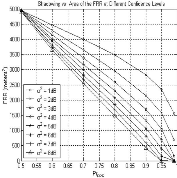
Figure 3 Illustration of the area of FRR vs. the level of confidence in the regenerator case under different levels of shadowing effect. Note:  $Pr_e^{ab} = 10^{-3}$ ,  $\gamma=4$ ,  $(P_c + P_{rec}(R))/\alpha_R = 0.1$ .
