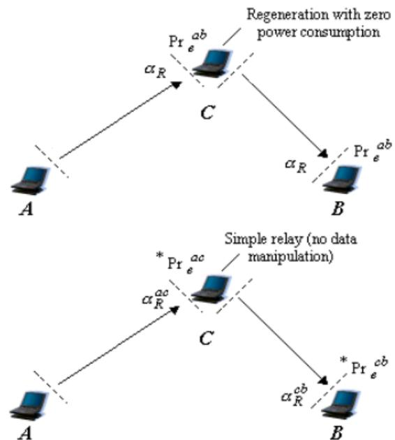
Figure 1 Illustration of the received signal power levels and bit error rates at receiving terminals in wireless transmission over (top) the regenerator (bottom) simple relay intermediate node.
