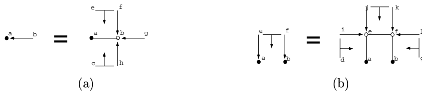
Figure 8: Graphical depiction of message update equations (Eq. 46; marginalize over nodes shown unfilled) for GBP using overlapping 4-node Kikuchi clusters. (a) Update equation for the single-index messages: M_a^b(x_a) = \alpha \sum_{x_b} \psi_b(x_b) \psi_{ab}(x_a, x_b) M_{ab}^{ef} M_b^f M_b^g M_b^h M_{ab}^{ch} . (b) Update equation for double-indexed messages (involves a division by the single-index messages on the left hand side).
