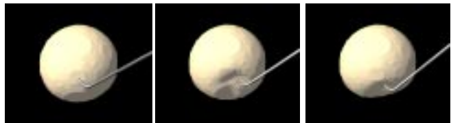
Fig. 7. Three still images from an interactive system in which a deformable 3D linked volume object is probed in real-time by a user controlled tool. Collisions between the object and the tool are detected using the occupancy map method and are used to calculate the object deformation. This object has size 40x40x40 and the occupancy map has size 200x200x200. Deformation of the sphere was performed using the algorithm presented in Section IV and the object was rendered by drawing triangles on the surface of the linked volume using OpenGL.
