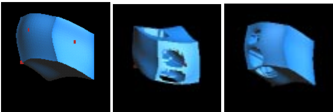
Fig. 22. Three still images from an interactive prototype system which models 3D object collisions, deformation, and carving. This object has size 20x20x20 and was rendered by drawing triangles on the surface of the linked volume using OpenGL. New triangles are generated interactively during object carving using the link structure.
