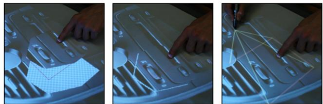
Figure 13. Coarse positioning of a selection with the hand (left and center). Pen in second hand allows pixel accurate transformation (right).
