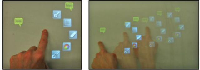
Figure 7. The menu command. One finger touch shows the menu (left). Dragging the menu (right).
