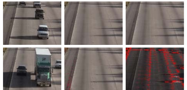
Fig. 5. EM update [4] vs. Bayesian update [5]. Left: Sample frames. Middle: First (top) and second (bottom) background layers of EM update. Right: Bayesian update result. EM update inaccurately blends distinct modes into identical layers. Bayesian update can identify separate layers, i.e. road and shadow modes. (Red means no layer)
