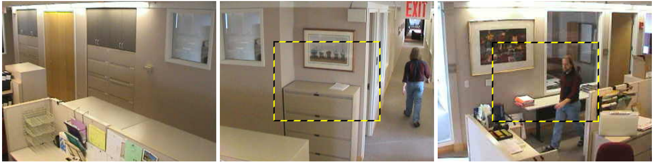
Figure 3: Example images from the validation run. Left: a miss. Middle: a hit. Right: a foveal hit, because the target is in the center 25% of the image (marked by the dashed frame for illustration).
