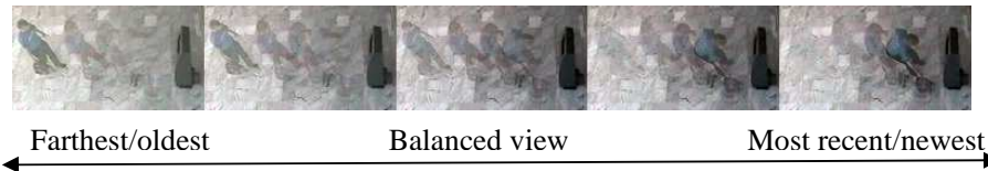
Fig. 2b. The transparency spectrum illustrating the effect of different weightings. The frame on the left emphasizes the (temporally) most distant frame; the frame on the right emphasizes the most recent. The balanced view falls in the center. The five sample frames from different points along the spectrum do not represent a video sequence; each frame is a composite image showing the different weighting schemes. Only one frame would be displayed within the Temporal Magic Lens.
