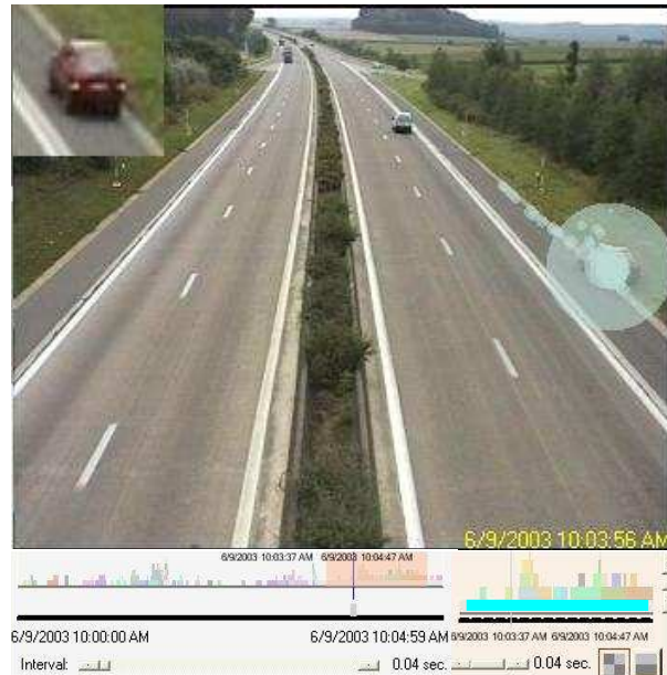
Fig. 3a. Object query - putting the cursor onto the object histogram shows the trajectory of the corresponding object in the video player. The object histogram spans the bottom of the application window. The long cyan bar at the bottom of the object histogram indicates an object present for a long period of time. Mousing over that bar brings up a thumbnail of that object (a red car), shown in the upper left-hand corner.
