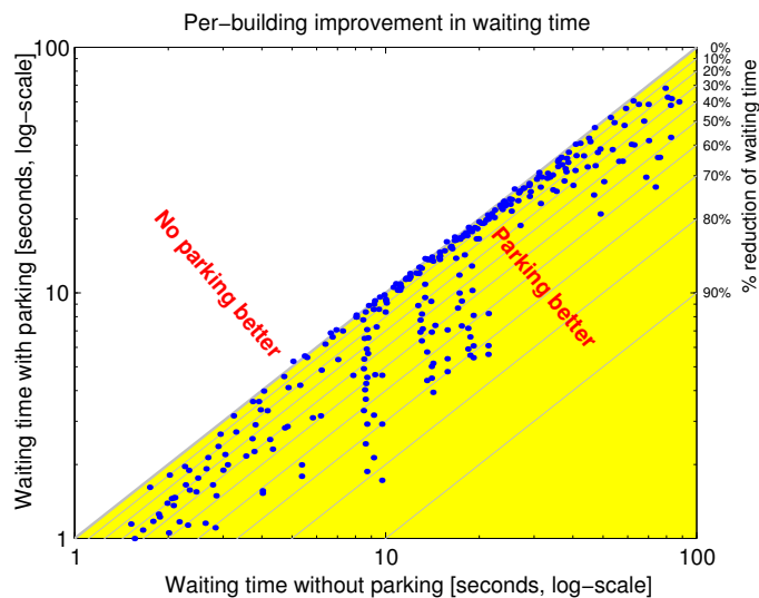
Fig. 3. Waiting times, in seconds, of two schedulers with and without parking, in both up-peak and down-peak traffic. Each dot represents an hour simulation in a different building type and arrival rate. Differences in waiting time in the range from 0 to 25 seconds are due to the parking controller, while differences above 25 seconds are due to the schedulers. (The parking controllers do not operate in this range, because there are no free cars to park for such building types, traffic patterns, and arrival rates.)
