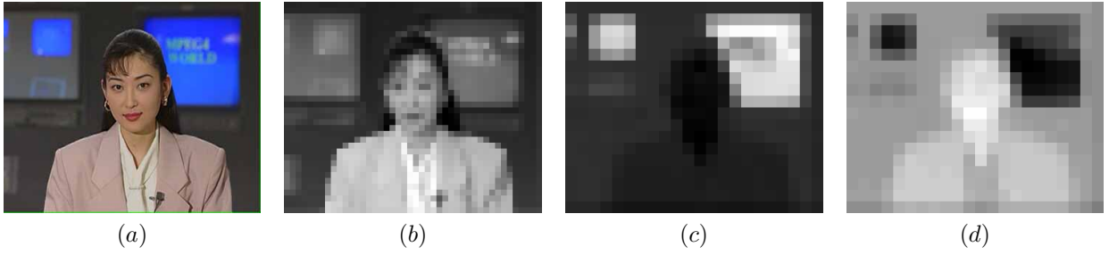
Figure 2. (a) Color image, (b) dc_y coefficients, (c) dc_u coefficients, (d) dc_v coefficients.
