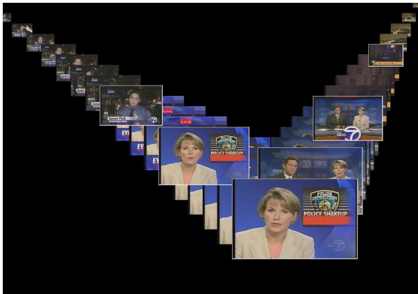
Figure 5: A video browsing interface in which key frames are drawn with a white border and are brought to the front of the drawing order.
