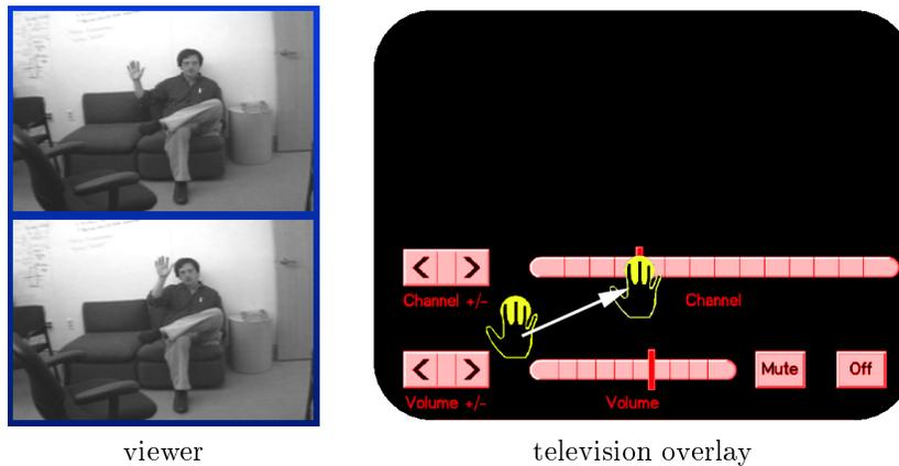
**Figure 4:** Adjusting a television set by hand signals. To get the attention of the television, the viewer raises his hand, palm toward the camera. When that gesture is detected, the television turns on, and a graphical overlay appears. A yellow hand tracks the position of the viewer's hand, and allows the viewer to use his hand like a mouse, selecting the desired menu item from the graphical interface. Normalized correlation with pre-stored hand templates performs the tracking.
