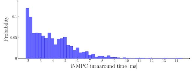
Fig. 6. Computation times per control time step of the iNMPC in Scalexio.
