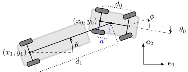
Fig. 1. Geometry of the considered SIT-system with a hitching offset,  $a$ .
