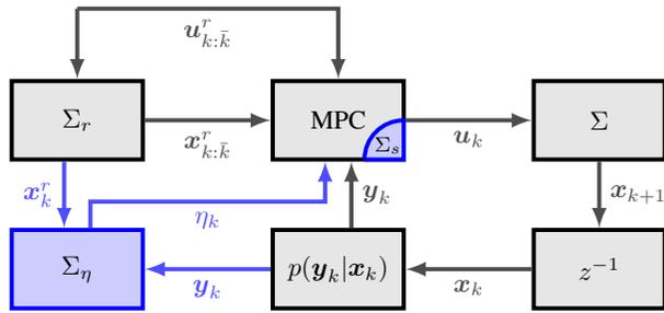
Fig. 2. Block diagram of a controlled system,  $\Sigma$ , driven along the trajectory of a reference system,  $\Sigma_r$ , by an MPC controller. The blue color indicates items that differ between a standard MPC and the proposed iNMPC. Specifically, the difference is in the computation of the integral term  $\eta$  in  $\Sigma_\eta$ , and the modification of  $\Sigma_s$  used in the MPC synthesis.
