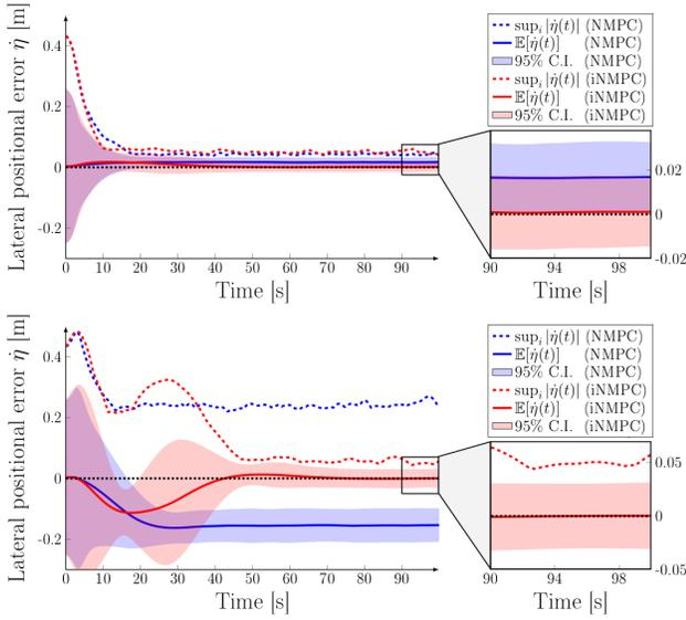
Fig. 3. Comparison of lateral positional tracking error,  $\eta$ , with the regular NMPC (blue) and the iNMPC (red), with statistics from  $10^3$  MC-executions. The  $2\sigma$ -interval is depicted along with the largest tracking error at every point in time over all of the realizations (dotted), with a zoom on the terminal errors. *Top*: Forward motion. *Bottom*: Backward motion.
