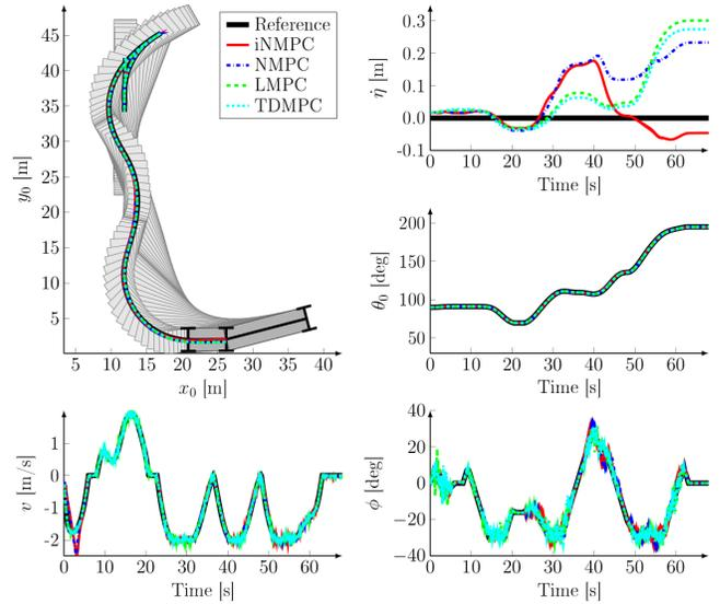
Fig. 4. One MC-simulation with the iNMPC (red), regular NMPC (blue), standard linear MPC (green) and TDMPC (cyan). *Top, left*: Configurations of the iNMPC response, and positional response  $(x_0(t), y_0(t))$  with all considered controllers. The wheelbases are drawn for the terminal configuration. *Top, right*: The lateral positional tracking error. *Center, right*: The trailer heading angle. *Bottom, left*: Velocity. *Bottom, right*: Steering angle.
