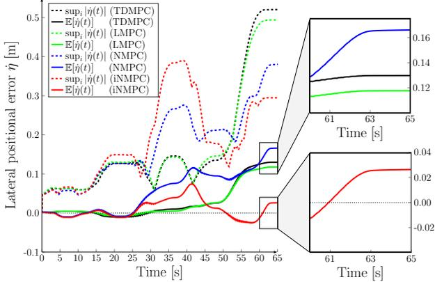
Fig. 5. Lateral positional tracking error,  $\dot{\eta}$ , with the iNMPC (red), regular NMPC (blue), LMPC (green) and TDMPC (yellow), summarizing the statistics from  $10^3$  MC-executions in terms of the mean error (full line) and the largest absolute error over all realizations (dotted).
