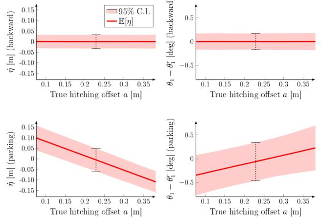
Fig. 7. The 95% confidence interval of the tracking error with the iNMPC as a function of the hitching offset in the controlled system,  $\Sigma$ , from  $10^3$  MC simulations. The dashed lines indicate the terminal errors when the hitching offset is known. *Top*: Backward motion. *Bottom*: Parking maneuver.
