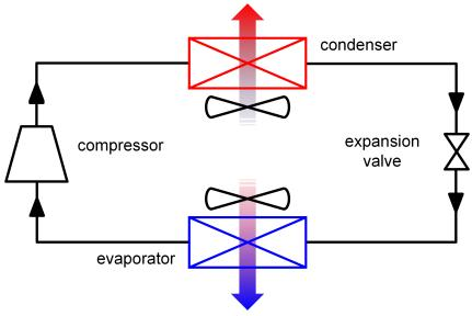
Fig. 3: Structure of a vapor compression cycle.
