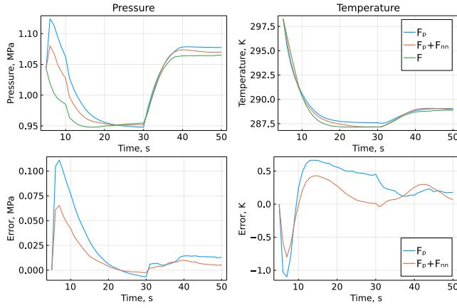
Fig. 4: Top row of plots shows comparison between the trajectory of the high fidelity VCC model ( $F$ ), the low fidelity model ( $F_p$ ) and the reconstructed using low fidelity physics-augmented neural networks ( $F_p+F_{nn}$ ) for states of one of the finite volumes. The bottom row shows corresponding errors calculated with respect to high fidelity VCC model ( $F$ ).
