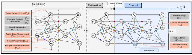
Fig. 2: Factor graph architecture for the simultaneous tactile estimator-controller
