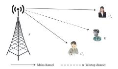
Fig. 1. System model consisting of a base station (S), two legitimate users  $(U_n \text{ and } U_m)$ , and an illegitimate eavesdropper (E).
