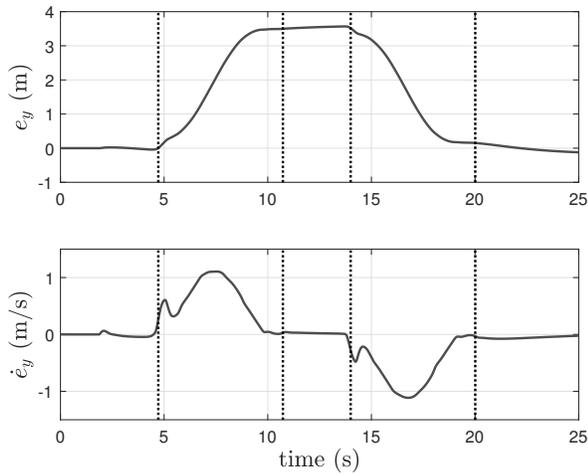
Fig. 4. Plots corresponding to driver-initiated lane changes: Position from reference lane (top) and relative rate of change of position (bottom); vertical lines signify transitions between modes
