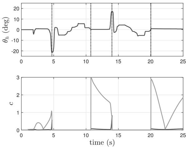
Fig. 5. Plots corresponding to driver-initiated lane changes: Steering wheel position (top) and cost of lane-keeping (bottom, dark) and cost of lane change (bottom, light); vertical lines signify transitions between modes
