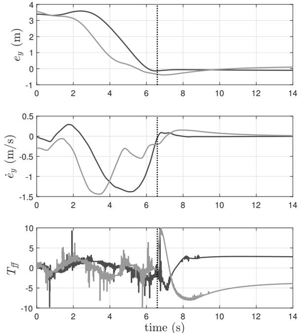
Fig. 3. Plots corresponding to autonomous takeover for nominal (dark) and alternative (light) control schemes: Position from reference lane (top), relative rate of change of position (middle), and dimensionless force-feedback command sent to the gaming wheel ( $\pm 10$  are saturation bounds); vertical lines signify a transition to autonomous mode
