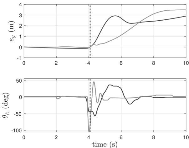
Fig. 6. Plots corresponding to manual takeover for nominal (dark) and alternative (light) control schemes: Position from reference lane (top) and steering wheel position (bottom); vertical lines signify transitions between modes
