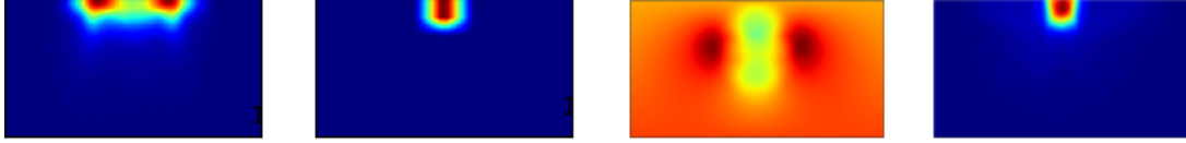
Fig. 2. From left to right: Irradiance field \hat{I} before tailoring; target irradiance pattern I ; height field z of the freeform after tailoring; irradiance pattern \hat{I} after tailoring.
