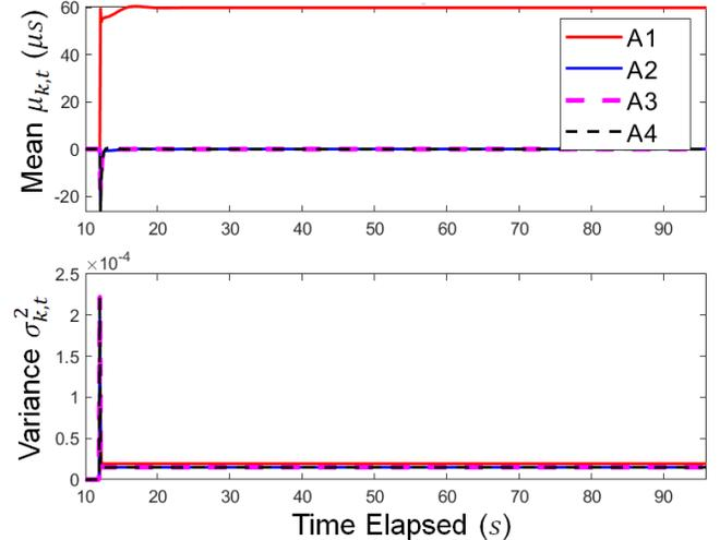
Fig. 7: Antenna-specific timing errors estimated during BP step, in particular its mean  $\mu_1$  and variance  $\sigma_1^2$ .
