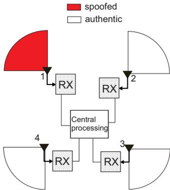
Fig. 1: Configuration of the proposed DMDA setup. Each directional antenna is provided with selective visibility by pointing it towards a different section of the sky, such that, not all the directional antennas can be spoofed simultaneously. Sector of circle represents the field-of-view of each antenna.
