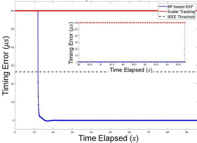
Fig. 6: Timing error estimated using the proposed BP-EKF algorithm, indicated in blue, is compared to that of the conventional scalar tracking scheme, indicated in red.
