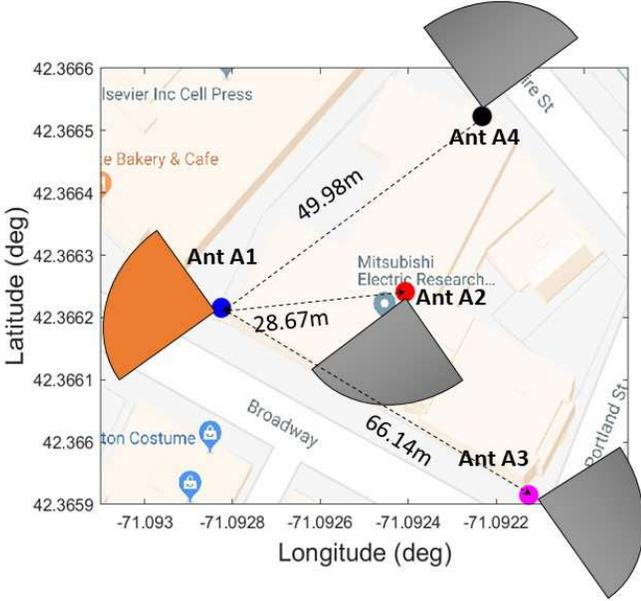
Fig. 4: Experiment setup consisting of four antenna-based DMDA with A1 antenna experiencing spoofing. The baseline information across antennas are pre-determined.
