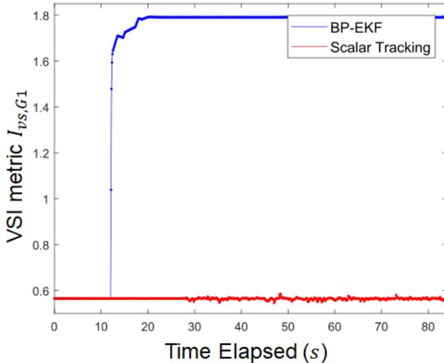
Fig. 8: Voltage Stability Index (VSI) of the G1 bus at the microgrid monitoring using two PMUs, one triggered via BP-EKF and the other via scalar tracking.
