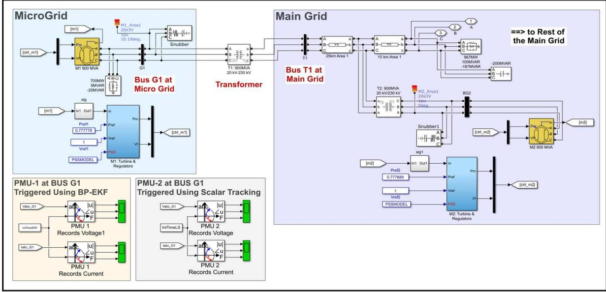
Fig. 5: The simulated grid setup consists of a microgrid which is connected to the main grid. The bus G1 monitors a critical node connecting the microgrid and the main grid. In the presence of meaconing, two PMUs are monitoring the bus G1, one of which is triggered using the BP-EKF algorithm and the other is triggered using the conventional scalar tracking scheme.
