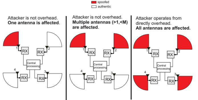
Fig. 2: Different spatial configurations of the attacker with respect to the proposed DMDA setup.
