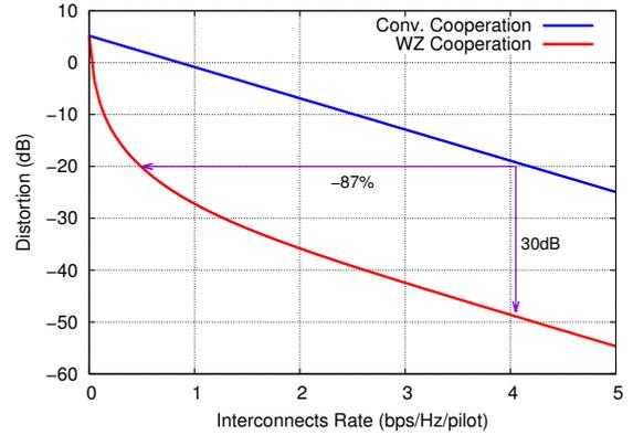
**Fig. 3:** Distortion of WZ-coded data representation as a function of interconnect bandwidth.
