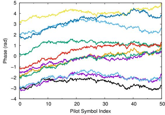
**Fig. 2:** Example of carrier phase changes for 11 superchannels ( $\Delta\nu = 1\text{MHz}$ ,  $\rho = 0.6$ , 32GBd, 1% pilot).
