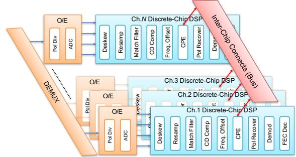
**Fig. 1:** Superchannel receiver using multiple discrete DSP chips and band-limited interconnects for cooperative MIMO processing.
