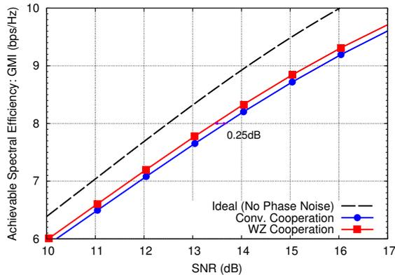
Fig. 6: GMI vs. SNR with cooperative CPE for an interconnect rate of 1 b/s/Hz/pilot.
