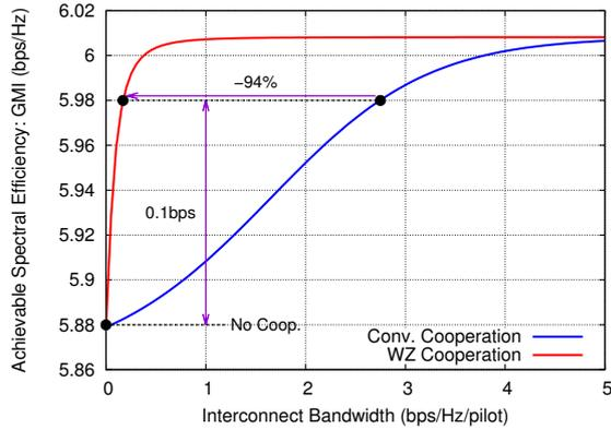
Fig. 5: GMI of DP-64QAM transmission with cooperative CPE as a function of interconnect bandwidth.
