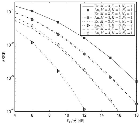
Fig. 7. ASER for several system setups. When  $K = 1$ , the ASER corresponds to the CP-SC system with selection combining.
