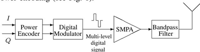
Fig. 1. An example of all-digital transmitter architecture.
