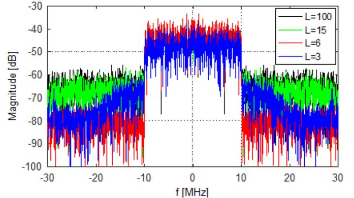
Fig. 5. Baseband spectrum of DSM-PWM output for various selection of DSM quantization levels.
