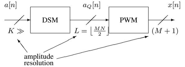
Fig. 4. Block diagram of the proposed DSM-PWM architecture.
