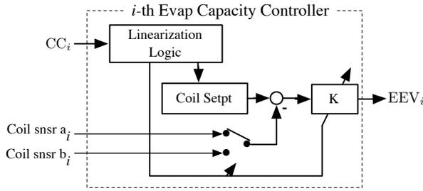
Fig. 4. Block diagram of the evaporator capacity controller used to control the refrigerant distribution in a multi-path heat exchanger and thereby modulate the cooling capacity.
