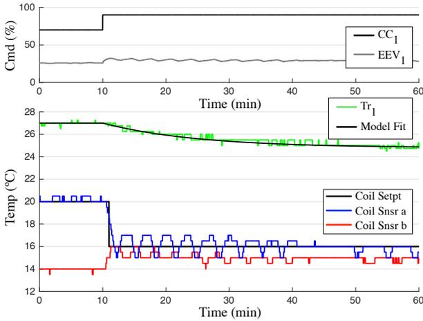
Fig. 5. A step change in capacity command results in a room temperature response to which a linear model is fit. Top: capacity command for zone 1 and the EEV position. Bottom: Coil setpoint for the selected heat exchanger path, and the two coil temperatures. The resulting zone temperature is also shown, as well as the response of a model fit to the transfer function from CC to Tr.
