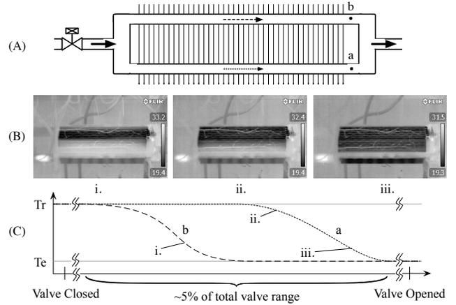
Fig. 3. (A) Multi-path heat exchanger with paths labeled ‘a’ and ‘b.’ (B) Infrared images of a multi-path heat exchanger for three different valve openings, i–iii. (C) Temperatures for paths  $a$  and  $b$  vary between the evaporating temperature  $Te$  and zone temperature  $Tr$  as the valve opening is changed. The three conditions represented by the IR images are indicated.
