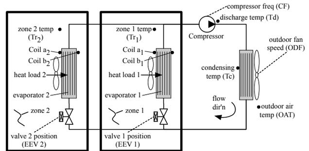
Fig. 1. Refrigerant piping arrangement of a multi-evaporator vapor compression system. Available sensors are shown as dots and control inputs are indicated with dashed lines.
