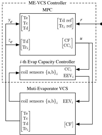
Fig. 2. Block diagram of the ME-VCS controller consisting of the capacity controllers for each evaporator coordinated by a model predictive controller.
