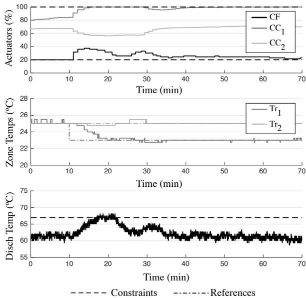
Fig. 7. Transient response using the capacity controller to drive zones to different setpoints. MPC selects inputs that simultaneously enforce constraints on CC input and Td output and results in zero steady state error in zone temperatures.
