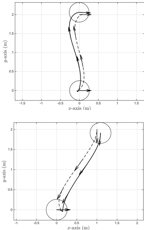
Fig. 3. Experimental results with robot trajectories (solid) and associated optimal paths (dashed) and initial positions, both  $(0, 0, 0)$ , and final positions,  $(0\text{m}, 2\text{m}, 0)$  and  $(1\text{m}, 2\text{m}, -\frac{\pi}{2})$ , of the ground robot (circles)
