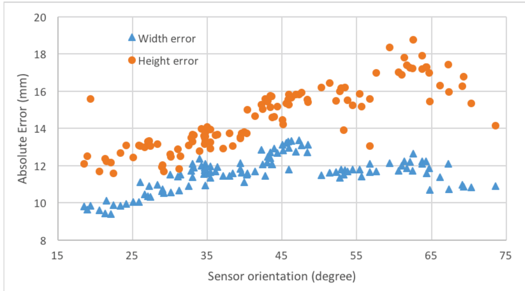
Fig. 8. Error of dimensions corresponding to sensor orientations for completed stair frames.
