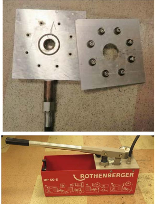
Figure 1: Pressure testing jig (above) and hydrostatic
