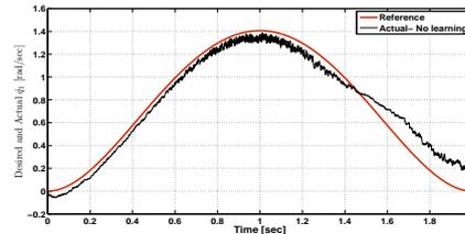
(b) Obtained vs. desired first angular velocity trajectory (No-learning)
