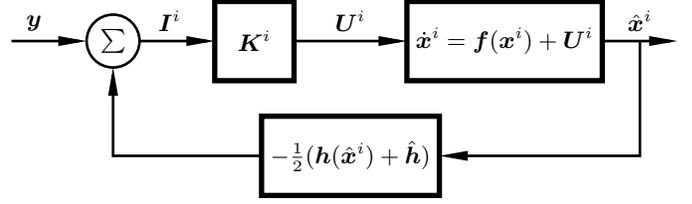
Fig. 1. Simplified block diagram of the FPF. It uses feedback gains  $\{\mathbf{K}^i\}_{i=1}^N$  to control the particles  $\{\mathbf{x}^i\}_{i=1}^N$ . This is in contrast to the conventional PF, where only the particles' weights are changed in the measurement update.
