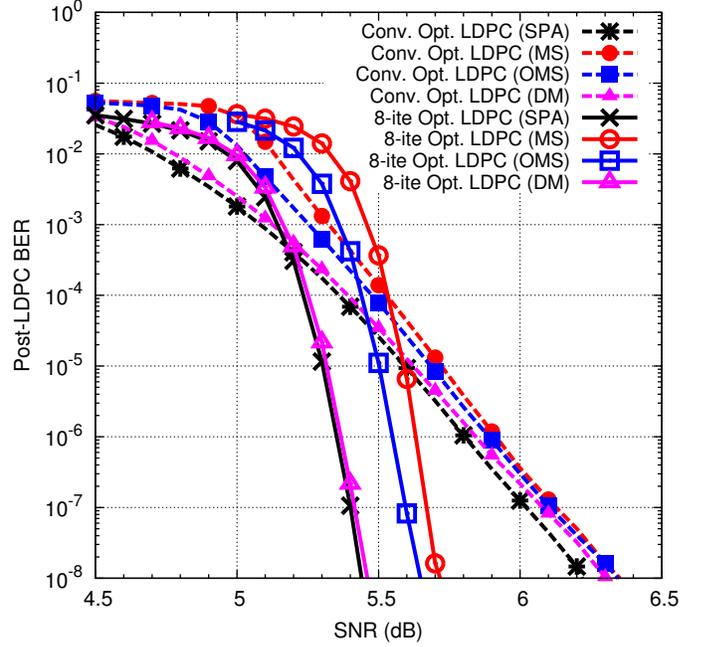
Fig. 6. BER performance of iteration-dependent LDPC code with different decoding algorithms for  $N_{\text{ite}} = 8$  (SPA: sum-product algorithm, MS: min-sum, OMS: offset min-sum, DM: delta-min).
