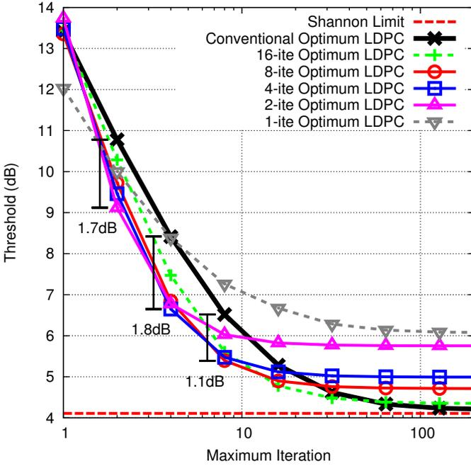
Fig. 3. Threshold vs. maximum iteration of iteration-aware LDPC codes with a code rate of  $R = 0.8$  for BICM with finite-iteration BP decoding.
