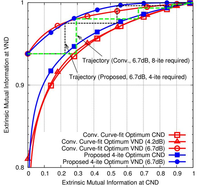
Fig. 2. EXIT curves of two irregular LDPC codes with a rate of 0.8: i) optimized degrees  $\lambda_\infty(x) = 0.150x^2 + 0.314x^3 + 0.536x^{12}$  and  $\rho_\infty(x) = 0.70x^{22} + 0.30x^{23}$  by conventional curve-fitting method and ii) optimized degrees  $\lambda_4(x) = 0.506x^5 + 0.494x^6$  and  $\rho_4(x) = 0.75x^{27} + 0.25x^{28}$  by iteration-aware trajectory method.
