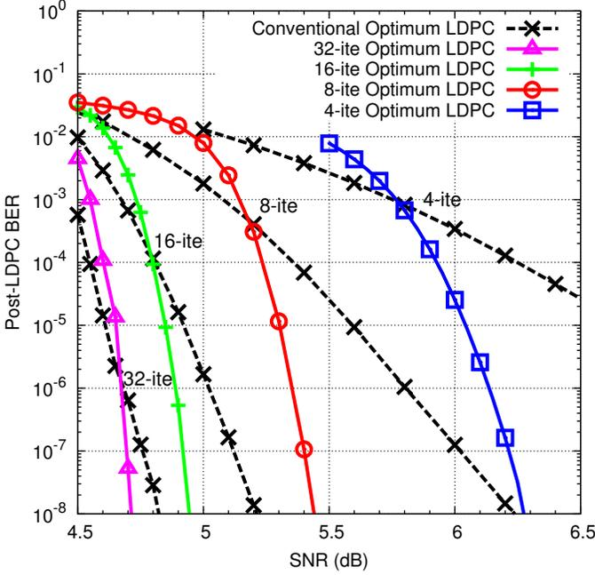
Fig. 5. BER performance of iteration-dependent LDPC codes with a code rate of  $R = 0.8$  for BICM with finite-iteration BP decoding.
