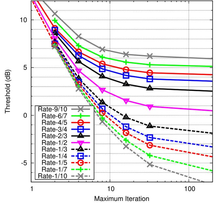
Fig. 4. Threshold of iteration-dependent LDPC codes with various code rates for BICM with finite-iteration BP decoding.
