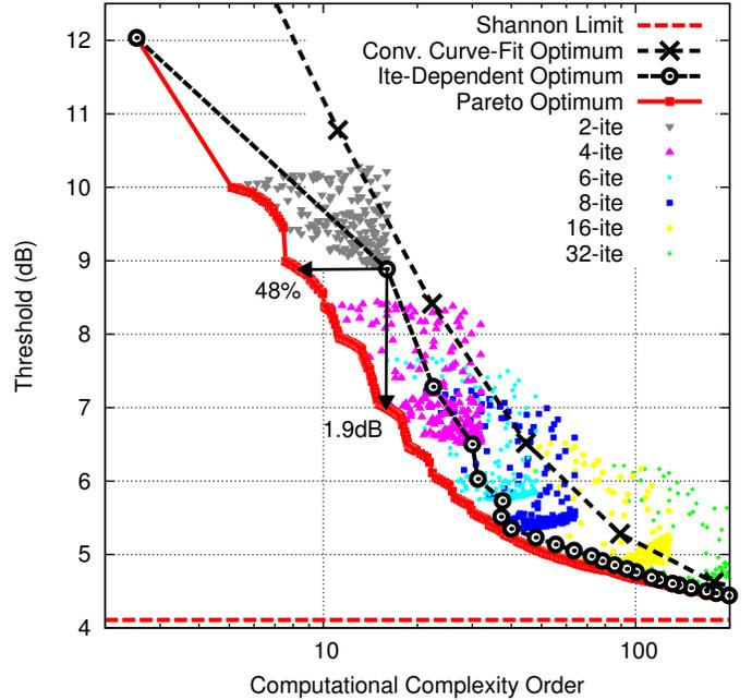
Fig. 7. Threshold vs. computational complexity of Pareto-optimal LDPC codes with a code rate of  $R = 0.8$  for BICM with finite-iteration BP decoding.
