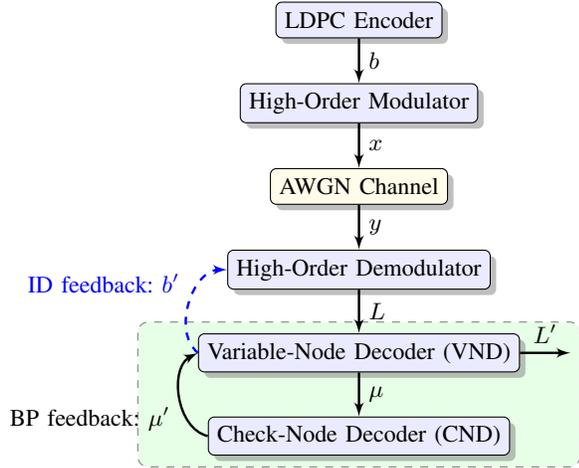
Fig. 1. Schematic of LDPC-coded modulation system for BICM.
