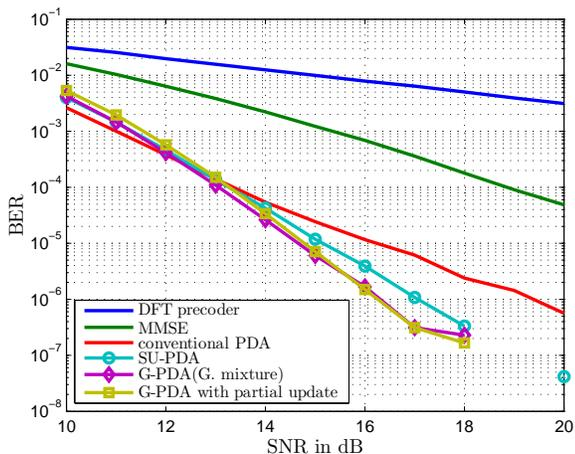
Fig. 7. Block size  $N = 32$ , QPSK modulation, measured channel, ten iterations. Remark: all algorithms yield the same performance with DFT precoder. All other plots correspond to identity precoder.
