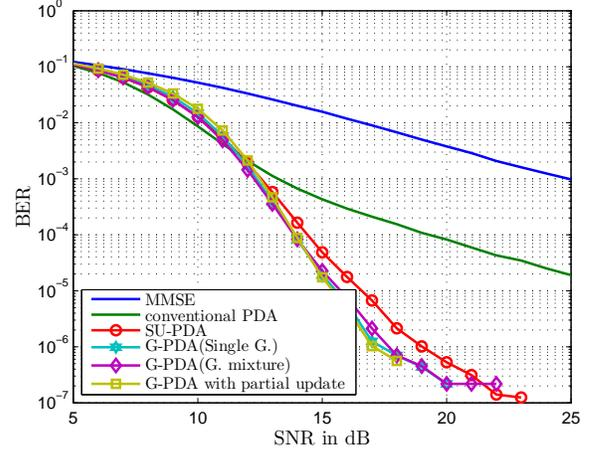
Fig. 2. Block size  $N = 16$ , QPSK modulation, DFT precoder, five-tap channel with fast fading, ten iterations. G-PDA with partial update is G-PDA with Gaussian mixture and no update on mixture weights.
