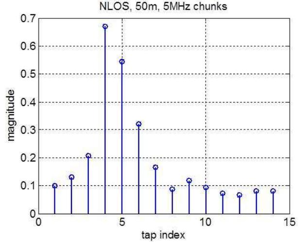
Fig. 5. One realization of a measured channel impulse response.
