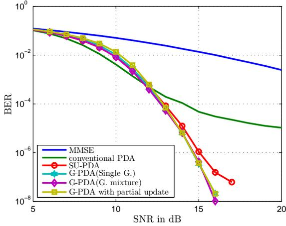
Fig. 3. Block size  $N = 32$ , QPSK modulation, DFT precoder, five-tap channel with fast fading, ten iterations. G-PDA with partial update is G-PDA with Gaussian mixture and no update on mixture weights.
