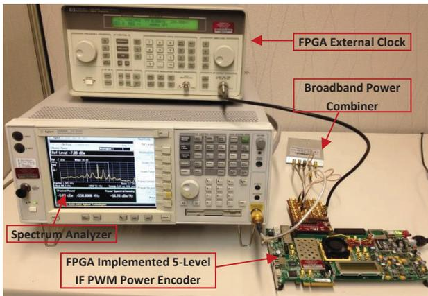
Fig. 6. Test bench for measuring the spectrum of FPGA implemented power encoder generated 5-level switching signals.
