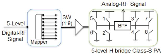
Fig. 5. FPGA control and topology of 5-level class-S PA.
