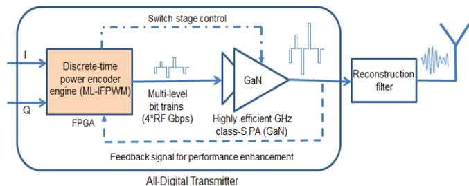
Fig. 1. All-digital transmitter architecture based on multi-level PWM power coding and highly efficient class-S digital PA.
