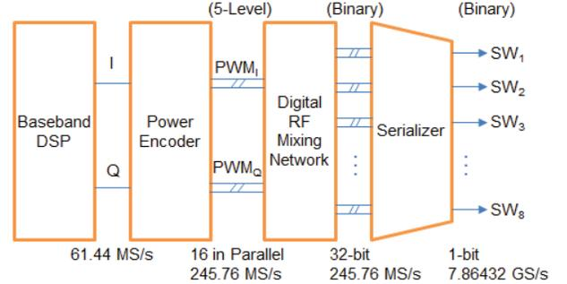
Fig. 4. All-Digital transmitter FPGA implementation for generating the switching signal for multi-level class-S digital PA.
