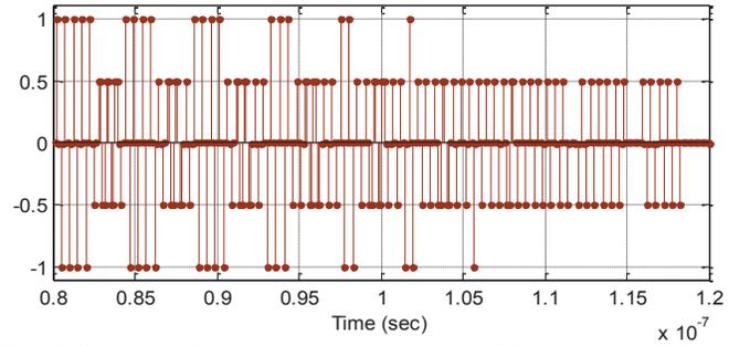
Fig. 3. Simulated 5-level discrete-time digital-RF out of encoder.
