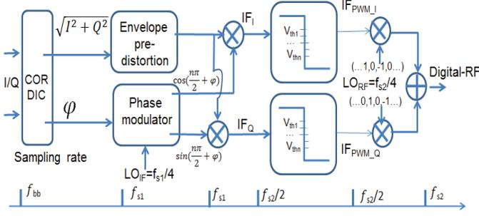
Fig. 2. Multi-level discrete-time IFPWM power coding diagram.
