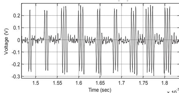
Fig. 7. Measured 3-Level final output from power encoder .
