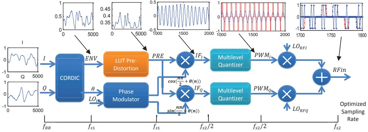
Fig. 2. ML-IFPWM power coding diagram.
