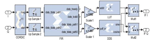
Fig. 5. Digital pre-distortion block diagram.
