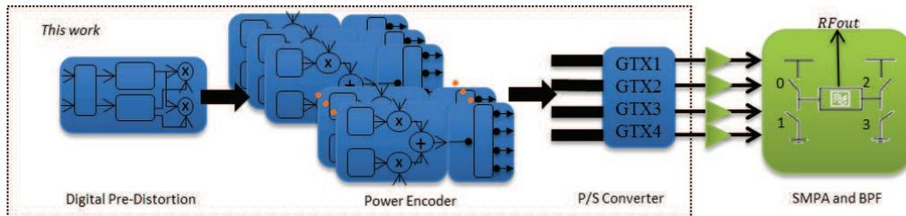
Fig. 4. System architecture diagram of All-Digital transmitter with FPGA implemented front end.
