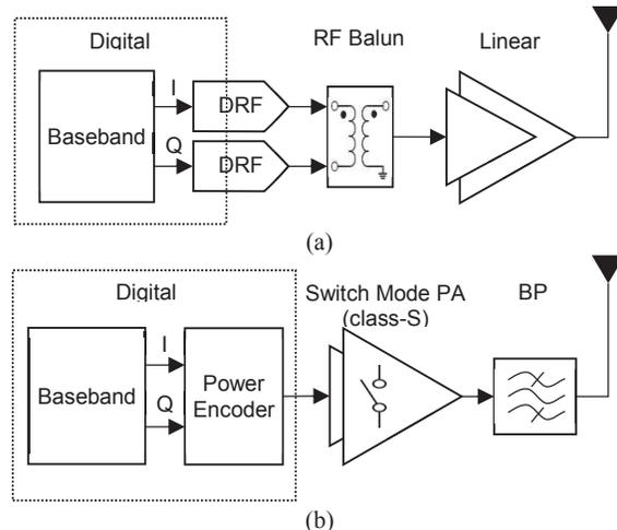
Fig. 1. Two digital-RF transmitter architectures based on (a) linear PA, and (b) switch mode PA, respectively.
