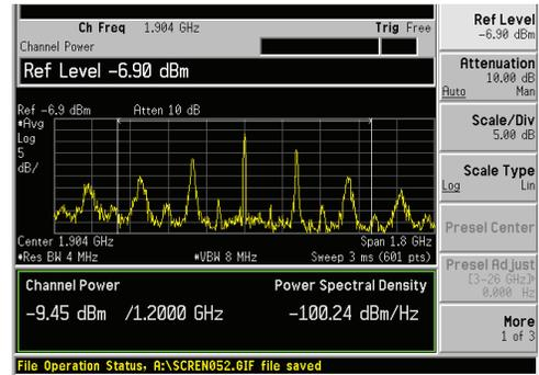
Fig. 8. Measured spectrum from output of power encoder .
