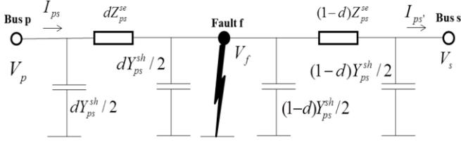
Fig. 3. Model of a line segment with a fault
