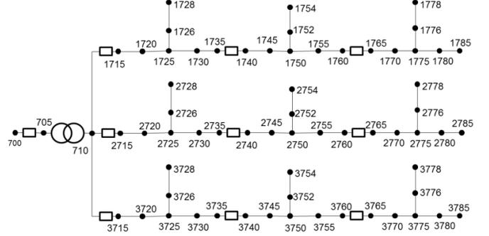
Fig. 4 A sample ungrounded distribution system
