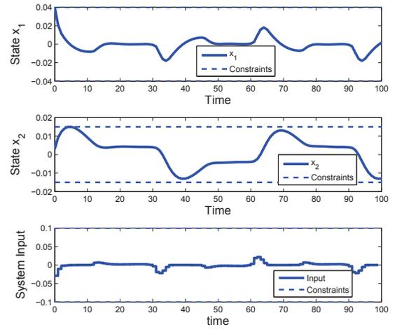
(b) State and input trajectories, and constraints
