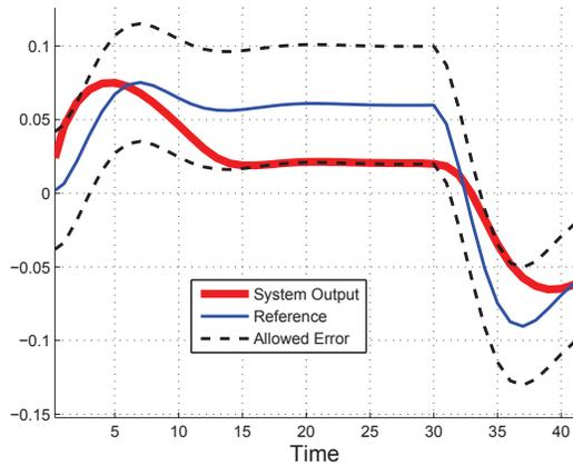
Fig. 2. Simulation of example system in closed-loop with the proposed controller. System output and reference in part of the simulation.
