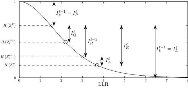
Fig. 1. Entropy as a function of LLR for an input symbol  $i$ . The contribution to the defined quantities is annotated, assuming that the symbol has not passed a new message, but received new information from its neighbors.
