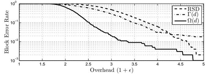
Fig. 6. Block error probability versus overhead for the simulated degree distributions.
