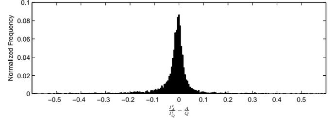
Fig. 3. Histogram of the difference between simulated  $I_A^l/I_Q^l$  from AWGN channel and theoretic  $A(L)/Q(L)$  from the BEC.
