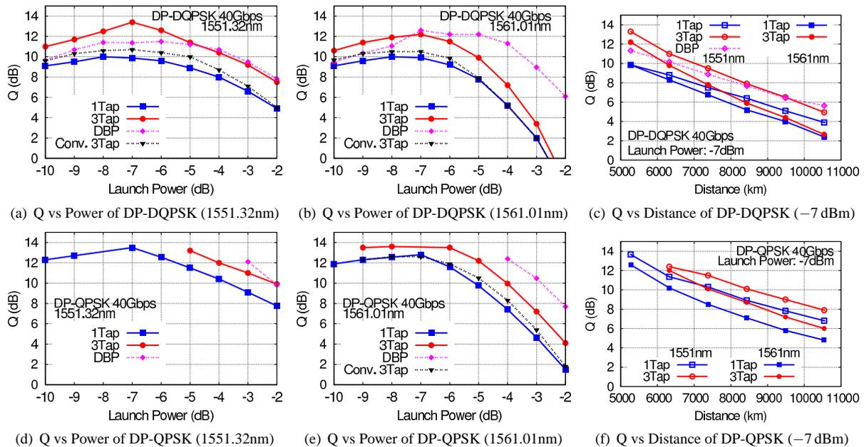
Fig. 2. Q-factor performance. “1Tap” denotes a phase compensation filter with no memory. “3Tap” denotes the proposed fractionally-spaced sequence equalizer with  $M = 3$  taps,  $N = 9$  excess window and  $P = 2$  oversampling. “DBP” denotes the original DBP with hundreds of SSFM iterations using manually optimized parameters. “Conv. 3Tap” denotes the conventional 3-tap statistical equalizer [6] without using the second-order statistics and oversampling.
