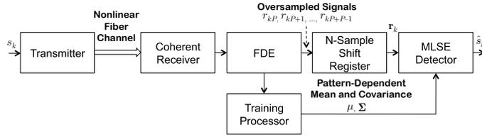
(a) Coherent system with fractionally-spaced statistical equalizer.
