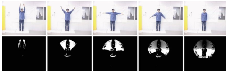
Fig. 2 Motion history images obtained by aggregating frame differences (© A. Ahad, 2010, Springer).
