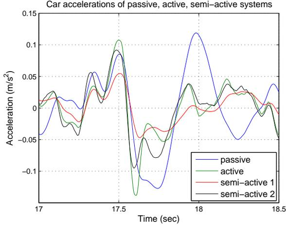
Fig. 3: Acceleration of passive, active, semi-active systems
