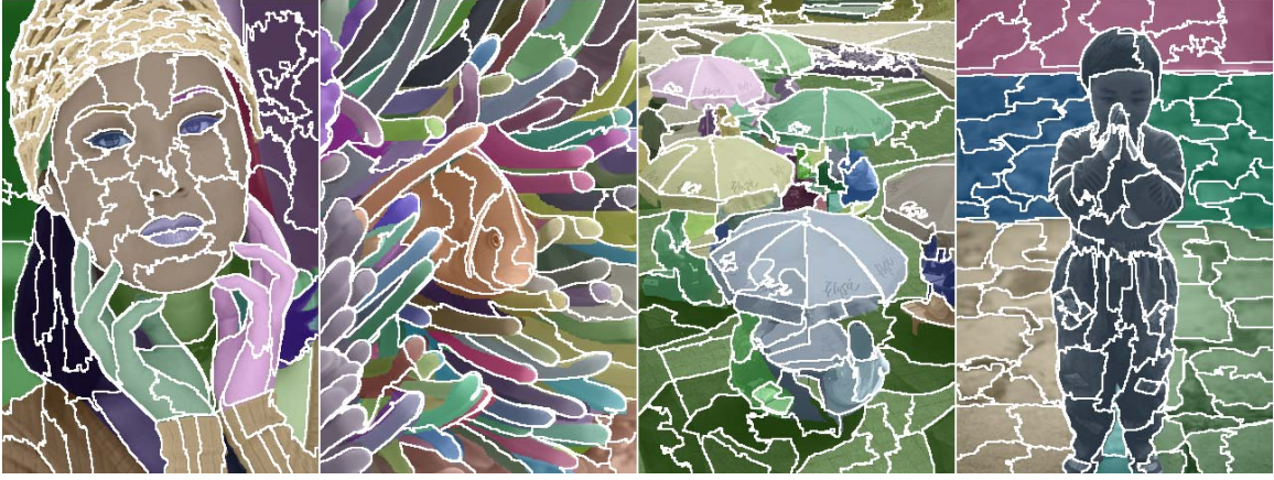
Figure 5. Superpixel segmentation examples. The images contain 100 superpixels. The ground truth segments are color-coded and blended on the images. The superpixels (boundaries shown in white) respect object boundaries and tend to divide an image into similar-sized regions.
