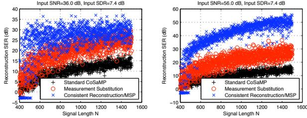
**Fig. 1.** Reconstruction Signal-to-Error ratio, for varying signal length  $N$ , with fixed sparsity  $K = 32$  and undersampling ratio  $M/N = 1/4$ . Results for two different input SNR are displayed.
