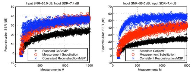
**Fig. 2.** Reconstruction Signal-to-Error ratio, for varying number of measurements  $M$ , with fixed sparsity  $K = 32$  and signal length  $N = 1000$ . Results for two different input SNR are displayed.
