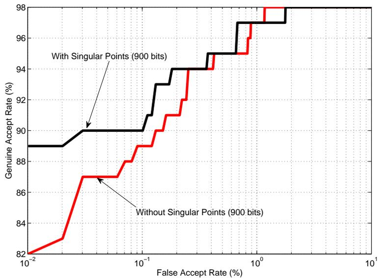
Figure 10. ROC curve with and without consideration of singular points (core and delta) for improved alignment.
