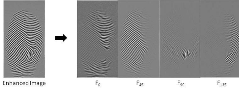
Figure 7. Four different filtered images are obtained from the enhanced image. One bit is extracted from each of these filtered images.
