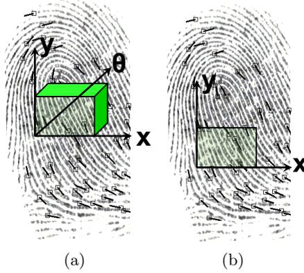
Figure 2. Example of a randomly chosen local aggregate regions in (a) 3D for minutia-based features and (b) 2D for ridge-based features.
