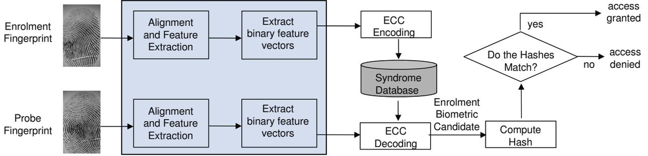
Figure 1. Schematic diagram for a syndrome-based secure fingerprint recognition system.
