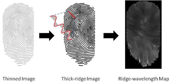
Figure 8. Extraction of ridge-wavelength features.
