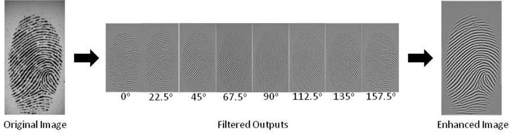
Figure 6. Enhancement procedure using Gabor filtering.
