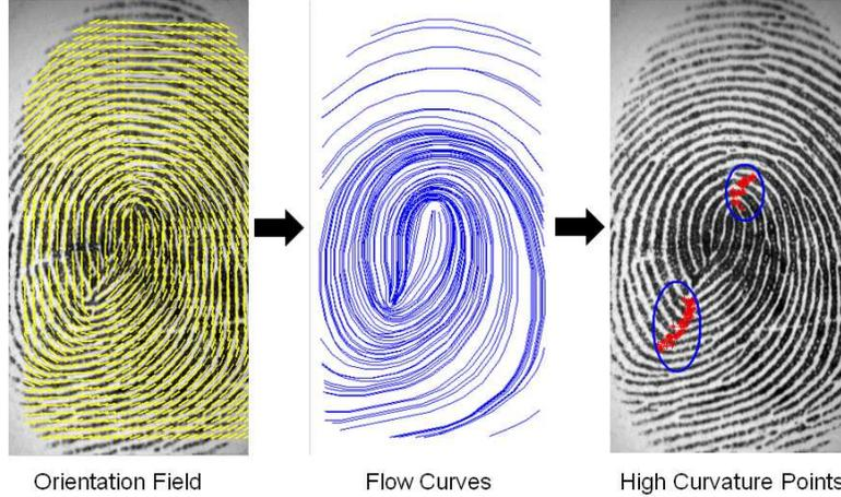
Figure 3. Extraction of high curvature points from a fingerprint. These high curvature points are stored on the access control device to facilitate secure alignment in the absence of the enrolled biometric sample.
