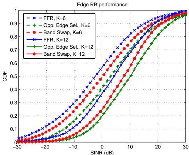
Fig. 6. Edge RB SINR distributions with 6 and 12 users per sector with  $RB_{\max} = 6$ .
