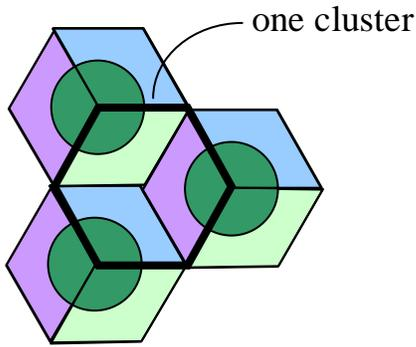
Fig. 2. Cluster in a sectorized cellular layout.
