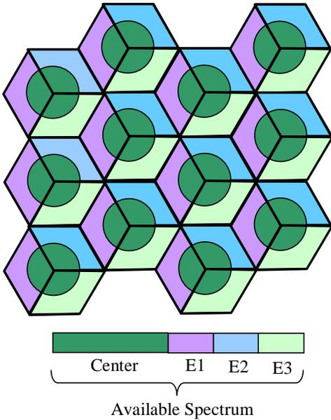
Fig. 1. Fractional frequency reuse layout for 3-sector cellular network.
