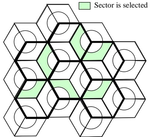
Fig. 3. Sample cellular scheduling layout on an edge RB.
