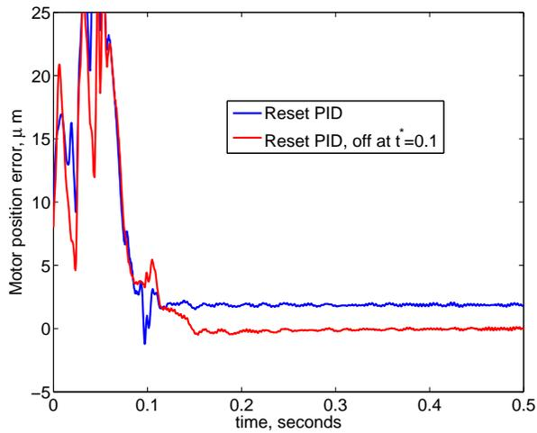
Fig. 8. Experimental positioning tracking error for a resetting PID controller with and without resetting turned off at 0.1 seconds.
