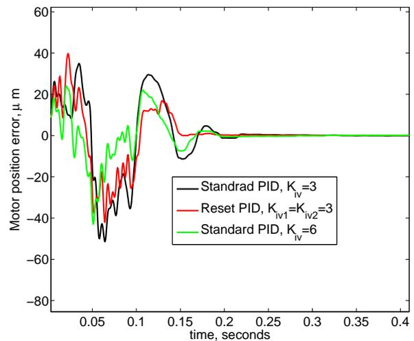
Fig. 7. Experimental positioning tracking error for 2 linear PID controllers and a resetting PID with 2 integrators.
