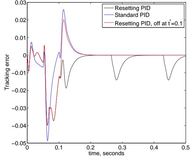
Fig. 3. Effect of constant disturbance on tracking error for different types of reset and non reset PID controllers; Turning the resetting off.
