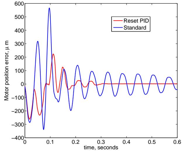
Fig. 6. Experimental positioning tracking error for an ill-tuned PID controller and its resetting counterpart.
