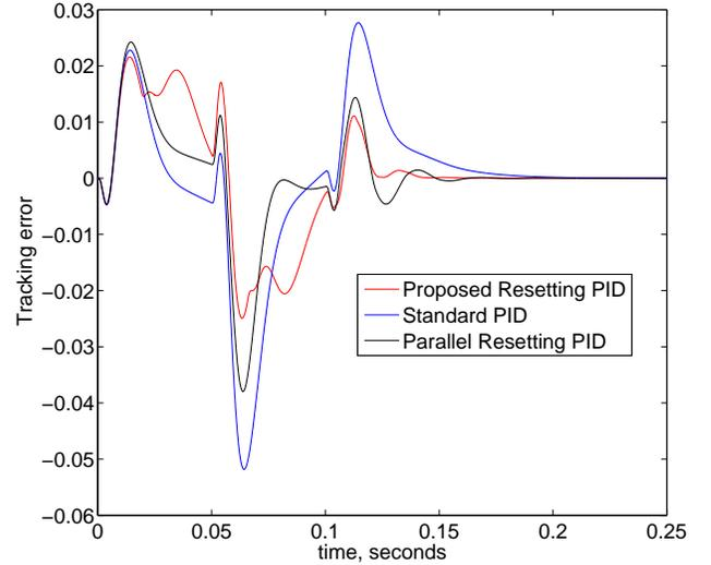
Fig. 1. Tracking error for series and parallel reset and non reset PID controllers.
