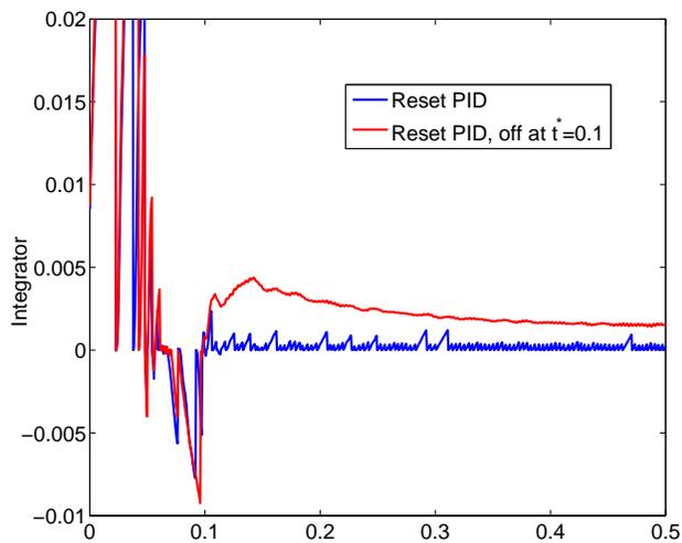
Fig. 9. Experimental integrator state for a resetting PID controller with and without resetting turned off at 0.1 seconds.
