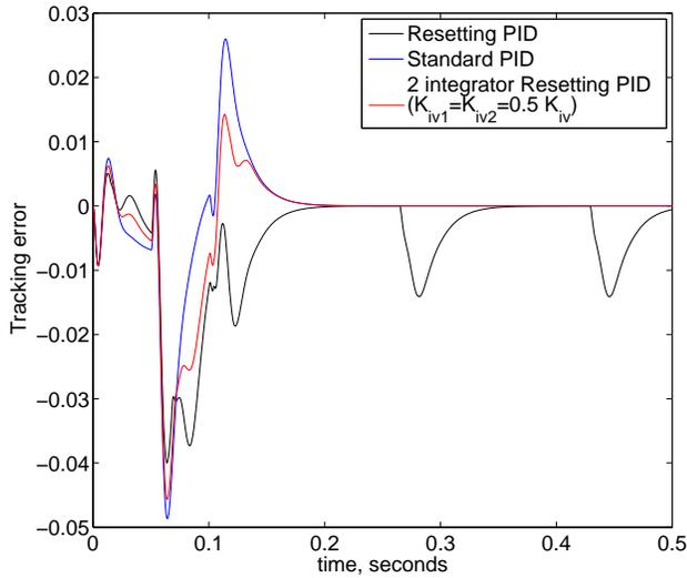
Fig. 4. Effect of constant disturbance on tracking error for different integral gain ratios for 2 integrator reset PID controller.
