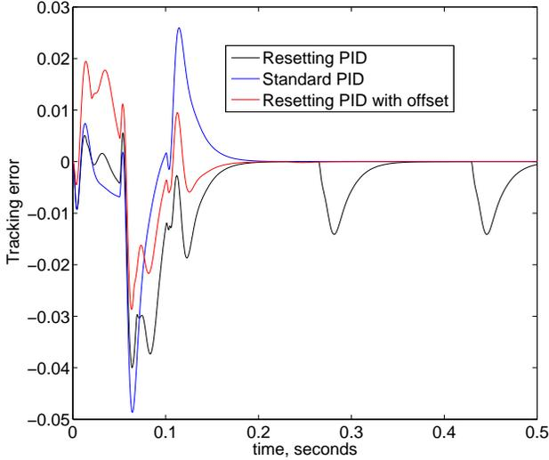
Fig. 2. Effect of constant disturbance on tracking error for different types of reset and non reset PID controllers; Resetting Offset.
