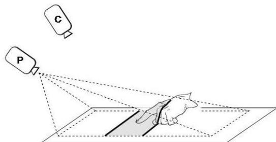
**Figure 2. Structured light in a projector-camera system distorted by the presence of a hand.**
