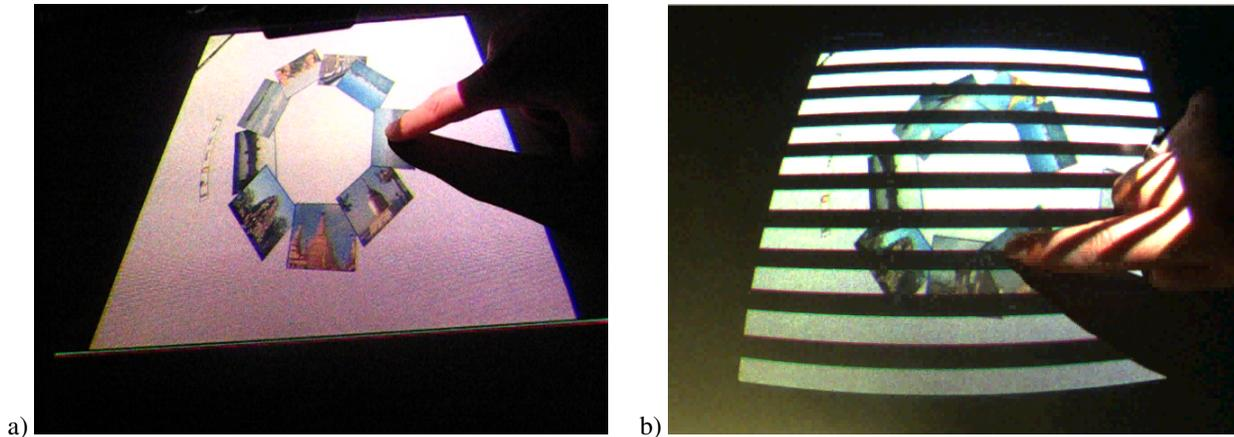
**Figure 3. Synchronized projector and camera to generate the stripes of the structured light. The figure shows the user's hand as seen by a human(a) and a camera(b).**
