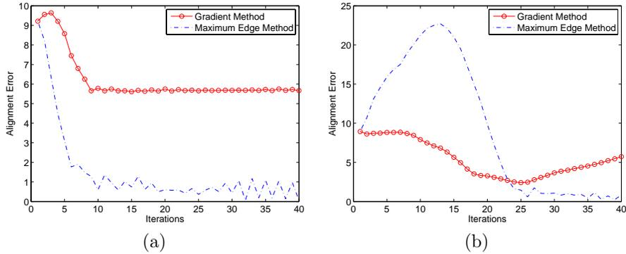
**Figure 4.** Rotation and translation estimation results for the multi-modality image registration. The IR image was rotated and translated by (a)  $(\theta = 0^\circ, \delta x = 6, \delta y = 7)$  (b)  $(\theta = 2^\circ, \delta x = 4, \delta y = 8)$  from the correct registration result. In both cases, our algorithm achieves correct registration results, while gradient method drifts away from the correct results.
