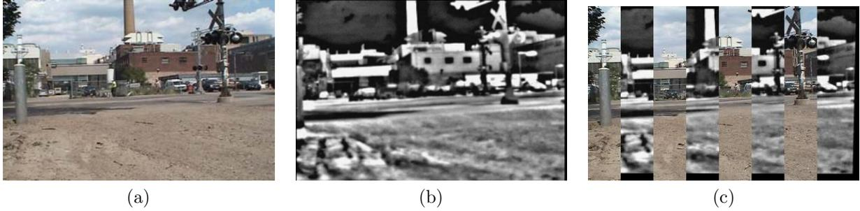
**Figure 3.** Multi-sensor Alignment. (a) Original visual image. (b) Original IR image. (c) Composite display after alignment. Original IR image was rotated and translated before alignment. Though the apparent visual difference and very different intensity values between the visible and IR images, our approach achieves good results on the experiments.
