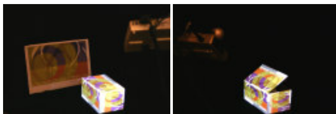
Figure 10: Projected augmentation on the box is attached to tags at the vertices, and so adapts automatically to the opening of the lid.
