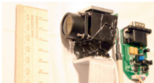
Figure 13: A micro-projector prototype we have built - to indicate the viability of designing a projector for truly handheld use. It is a 1-inch cube using an LED and LCOS imager to create a color animated projection at a distance of about 12-inches.
