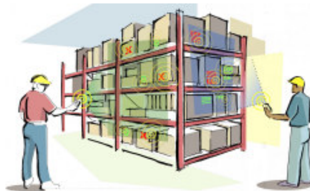
Figure 1: Warehouse scenario. A user directs a handheld projector at tagged inventory, with communication mediated by two channels – RF and photo-sensing on the tags. The user sees a projection of the retrieved tag information collocated with the physical objects, and performs a desktop-like interaction with the projection. A second user performs similar operations, without conflict in the interaction because the projector beams do not overlap.
