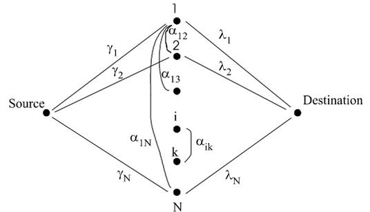
Fig. 1. System setup with source, destination, and  $N$  parallel relays. Channel gains between source to the  $i$ -th relay,  $i$ -th relay and the destination, and  $i$ -th and  $k$ -th relays are denoted by  $\gamma_i$ ,  $\lambda_i$ , and  $\alpha_{ik}$ , respectively.
