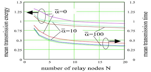
Fig. 4. Mean transmission time and mean expended energy for the asynchronous protocol as a function of the number of available relay nodes. Mean link gain between the relay nodes  $\bar{\alpha}$  is 0, 10, and 100.  $\bar{\gamma} = \bar{\lambda} = 10$ .
