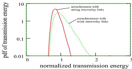
Fig. 5. Pdf of transmission energy with  $N = 10$  relay nodes for weak and strong inter-relay links.  $\bar{\gamma} = \bar{\lambda} = 10$ .
