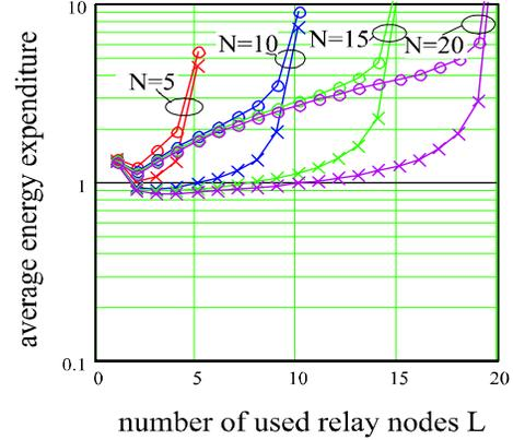
Fig. 2. Mean energy expenditure as a function of the number of active relay nodes  $L$  for different numbers of available relay nodes,  $N$ . Lines with crosses: multiple fountain codes (mutual-information-accumulating receiver). Lines with circles: single fountain code (energy-accumulating receiver).  $\bar{\gamma} = \bar{\lambda} = 10$ ,  $H_{\text{target}} = 1$ .
