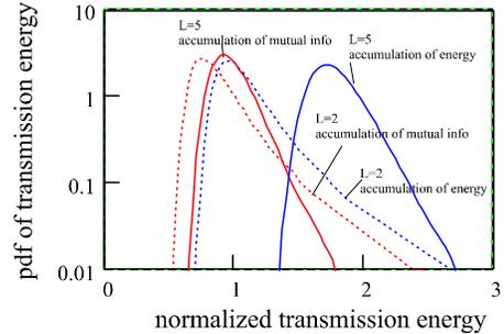
Fig. 3. Pdf of transmission energy for  $N = 10$ ,  $L = 2$  and 5,  $\bar{\gamma} = \bar{\lambda} = 10$ .
